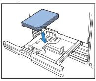
Move the guides against the edges of the paper, and push the lever to lock.
