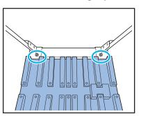
2 Fit the holes of the stacking tray on top of the knobs on the carriage.
