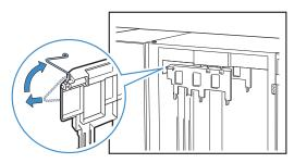
2 Lift the back corrugator while pressing it toward the machine (to the left).
