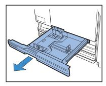
Push the locking lever (in back) to unlock the guides. Holding the front tab, spread the guides fully apart.
