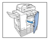
Remove the ink cartridge identified as empty.
