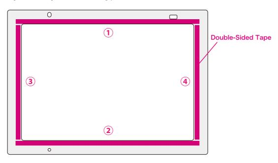
\*Make sure that the double-sided tape does not cover the holes.
