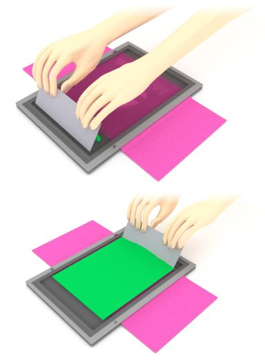
Replacing the substrate after each print enables consecutive printing.
