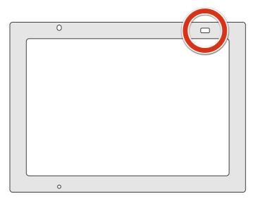
Apply double-sided tape in number order on the areas shown below on the frame. Do not peel off the protective backing yet.
